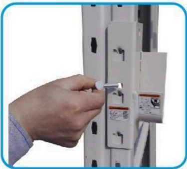
Safety Pin Locks Axle Bracket
